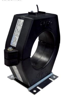
In case of earth fault in a three-phase network, a current occurs due to the displacement of the neutral point. This current is implemented with a specific ratio in the output of the sensor. Therefore the system enables to detect fault and short-circuit currents.
